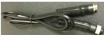
Camera extension cable. Male pin side is the camera end. Female end with tightening collar goes to Monitor or DVR.
